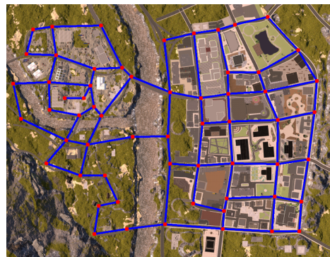
Fig. 1: Polypixel, a simulated urban environment used for our experiments (as seen in [7]), with its graph-based abstraction superimposed. Vertices show locations where a task has been assigned to one or more robots of a heterogeneous team. Edges represent travel paths between two locations.
